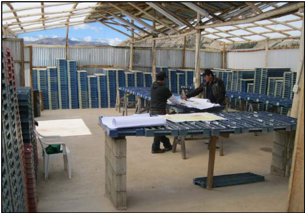
Figure 12.2 Drill Core Logging and Storage Facility (inside)
