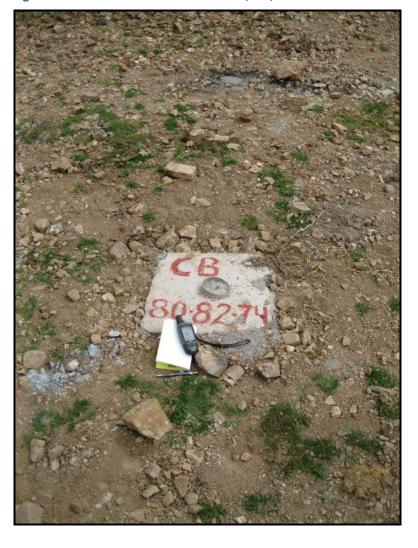
Figure 12.13 Drillhole Collar for CB-80, -82, -74
