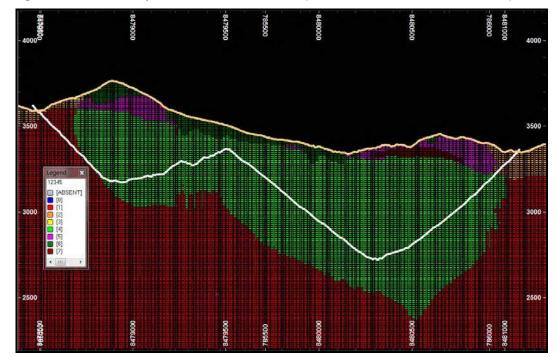
Figure 14.34 Conceptual Pit Shell Cross-section (south-southwest to north-northeast)
