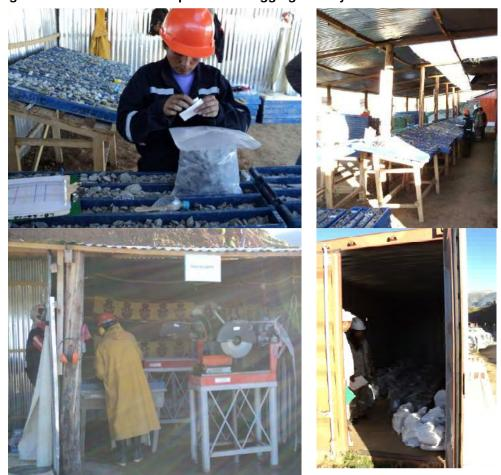
Note: Photographs are (clockwise from top left): Sampling fracture drill core, core logging benches, cutting area, and container for storage of samples to be dispatched to the laboratory and control materials. Photographs taken by Amec Foster Wheeler, 2012.
