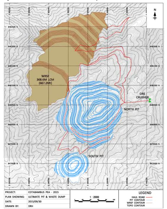
Figure 16-7: Ultimate Pits and Waste Rock Facility
