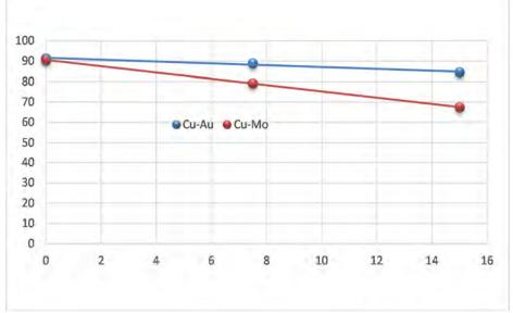
Figure 13-1: Effect on Cu Rougher Flotation Recovery vs Oxide Blending (wt%)
