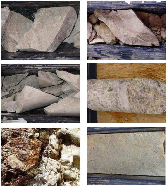
Note: Drill core is 8 cm wide. Clockwise from upper left: quartzite with bedding laminations at mm scale; delicate bedding features are offset along fractures; altered Main Porphyry with sulphide mineralization; quartz aphyric Late Porphyry; altered sediments (left) in contact with Main Porphyry (field of view is 4 m wide); fine grained lutite.
