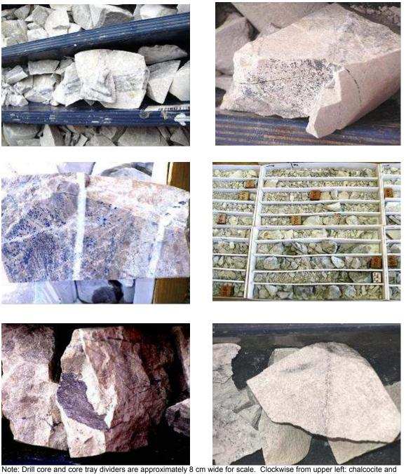
Note: Drill core and core tray dividers are approximately 8 cm wide for scale. Clockwise from upper left: chalcocite and quartz filled fractures in quartzite; chalcocite coating a fine late fracture in weakly altered quartzite; intense fracturing and sooty chalcocite mineralization associated with faulting: primary chalcopyrite mineralization in fractures below the secondary sulphide zone; molybdenite mineralization on fine fractures; chalcocite on fracture surface and in quartz veins.
